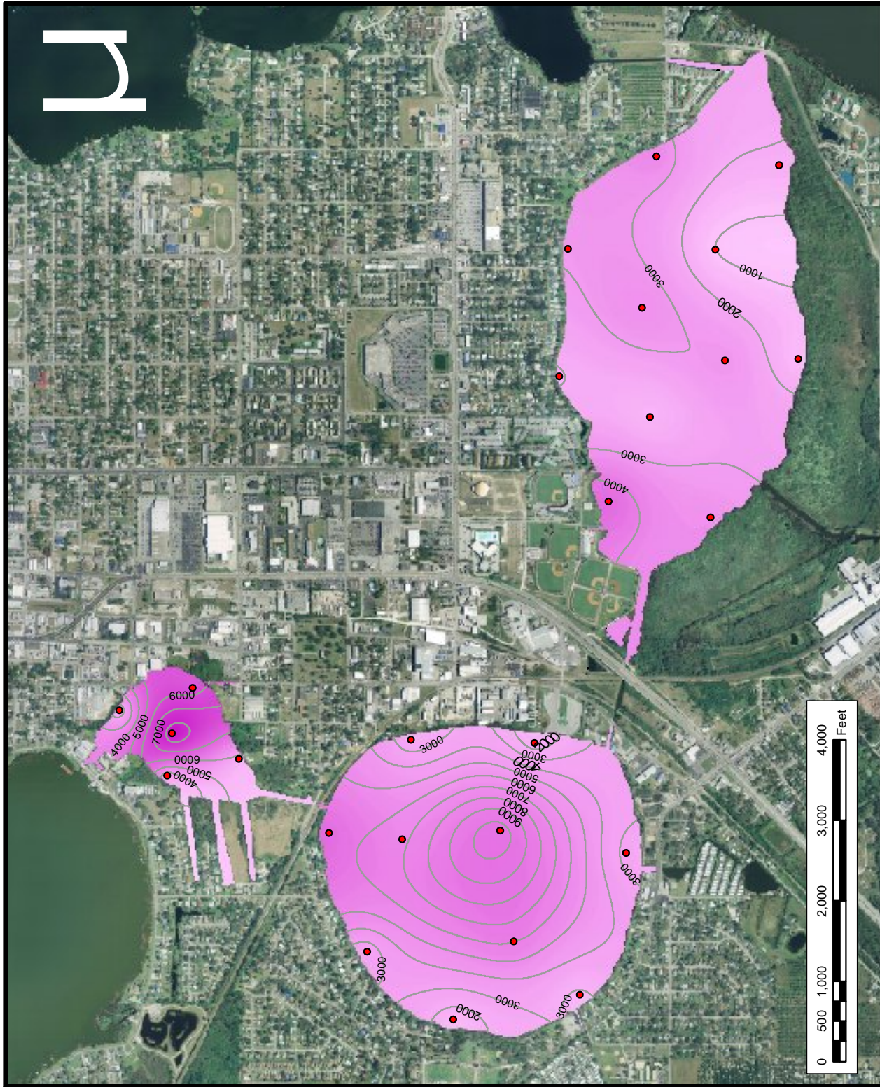
Figure 5-13. Mean Annual Isopleths of Total Nitrogen Concentrations in Groundwater Seepage Entering Lakes May, Shipp, and Lulu.
