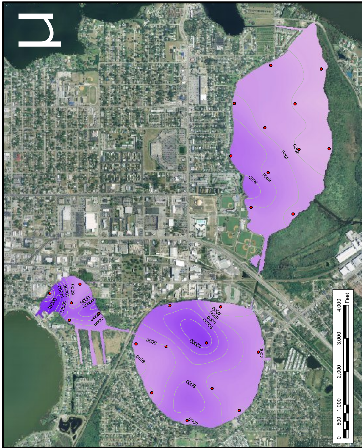
Figure 5-15. Isopleths of Annual Total Nitrogen Flux in Groundwater Seepage Entering Lakes May, Shipp, and Lulu.
