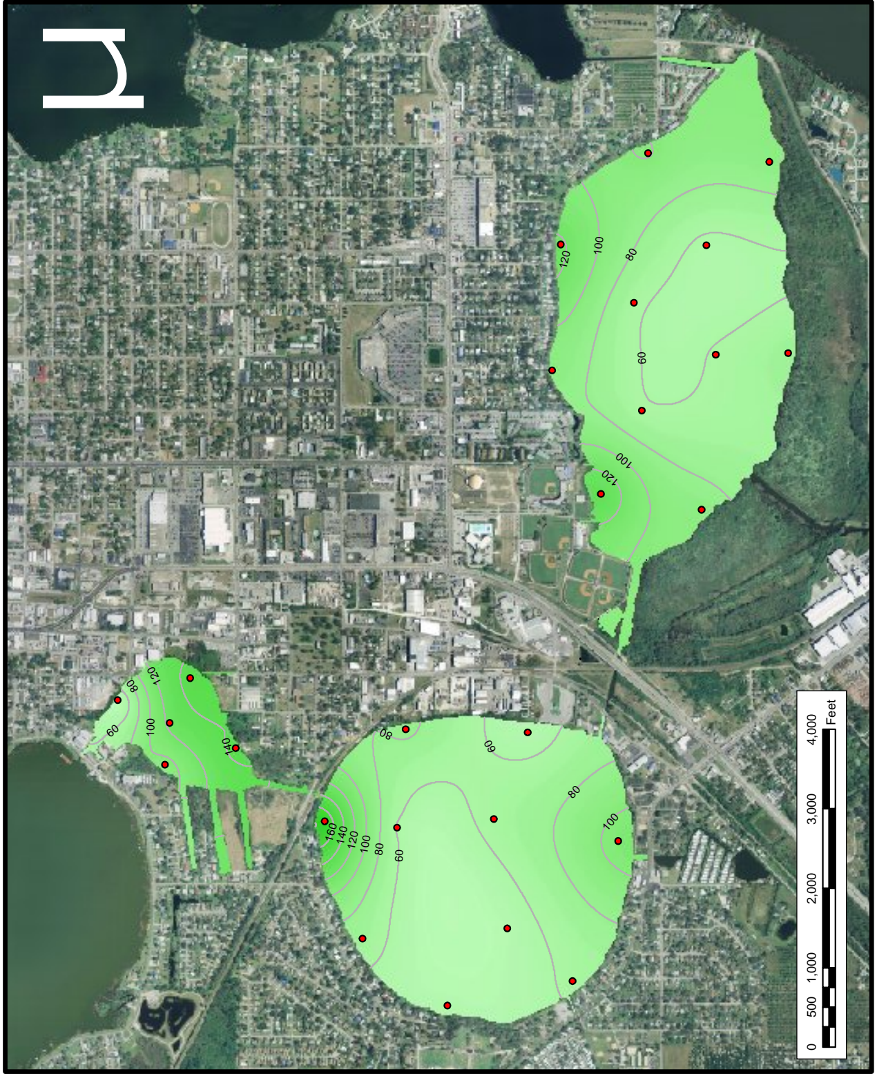
Figure 5-11. Estimated Mean Annual Alkalinity Concentrations (mg/l) in Groundwater Seepage Entering Lakes May, Shipp, and Lulu.
